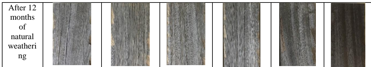
Figure 1. Thermally modified Eucalyptus globulus wood samples before and after 12 months of natural weathering.
