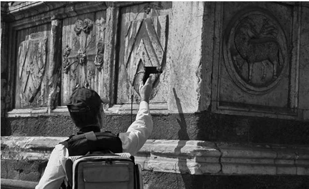
Fig.1: Acquisition of the VNIR/SWIR spectra from the Aveli tombstones using an ASD FieldSpec FR Pro spectrometer by Analytical Spectral Devices
