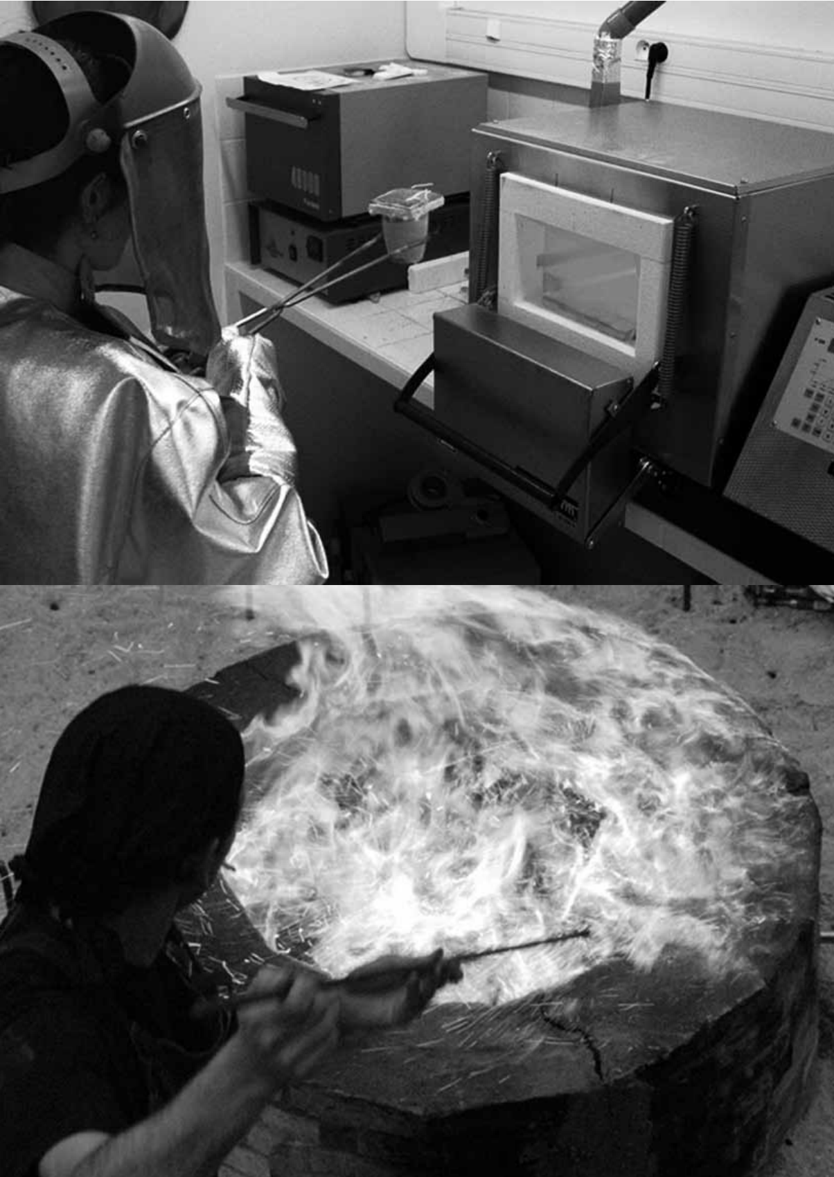
Fig. 1: Main components of the multiscale experimental set-up showing one electrical laboratory furnace as part of the in-door experimental platform (up), and a wind-powered furnace at the out-door experimental platform of Barys, Belgium (down)
