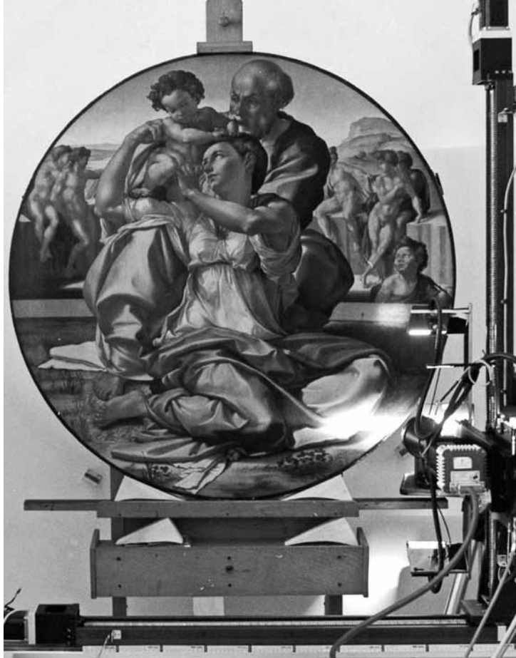
Fig.1 An application of the IFAC-CNR hyper-spectral scanner to the painting "Sacra Famiglia", or "Tondo Doni", (1504 -1507 ca.) by Michelangelo Buonarroti, belonging to the collection of the Uffizi Gallery (Florence).
