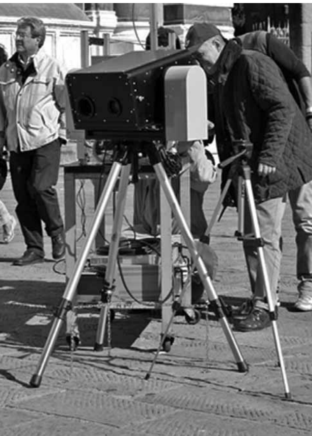
Fig.2: Monitoring campaign in Santa Maria Novella square using a Selex Galileo Multisensor Hyperspectral System (SIM-GA).
