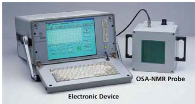
Figure 6.16: Hand-held NMR device for one-sided access.
