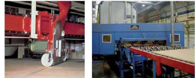
Figure 1.37: Diagonal saw for cut to length panels after continuous hot pressing (Metso Panelboard).
