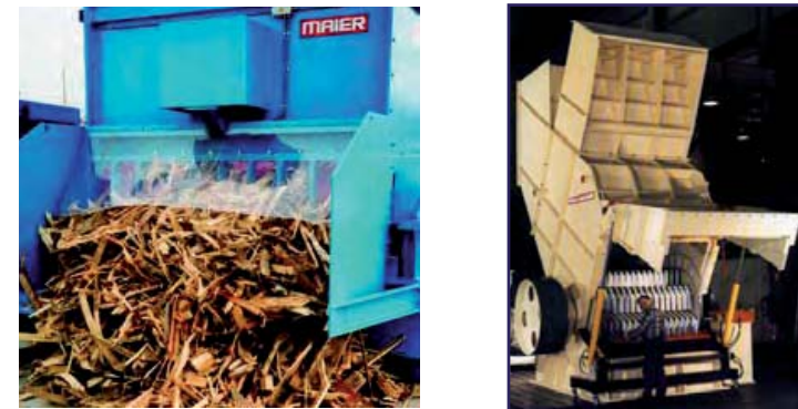
Figure 1.11: A hammer mill (Maier and Pallmann).
