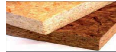
Figure 8.5: Particle board made of untreated and thermally modified chips of spruce ( Picea abies ).
