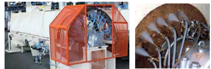
Figure 1.56: Dry fibre blender with open in-feed and spraying nozzles ring (IMAL).
