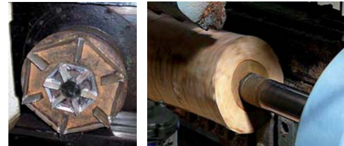
Figure 1.65: Left one of many chuck designs and right the chucks inserted in the log ends.
