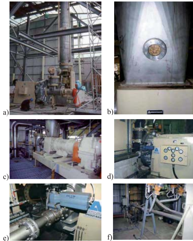
Figure 1.53: The main parts of a defibrator: a) tube, b) window, c) plugging screw, d) main engine, e) blow pipe, f) resin injection.
