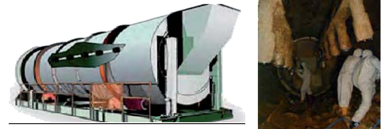
Figure 1.47: Drum resination of strands using atomizing discs (Metso Panelboard).
