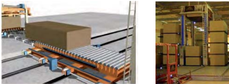
Figure 1.42: Full automatic intermediary storage system based on chariots (Metso Panelboard).
