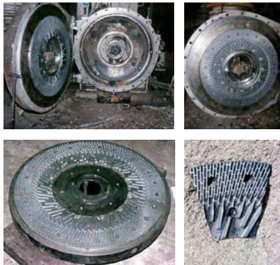
Figure 1.55: Photographs of the discs and segments found inside of a typical pressurised refiner used to make MDF fibre.
