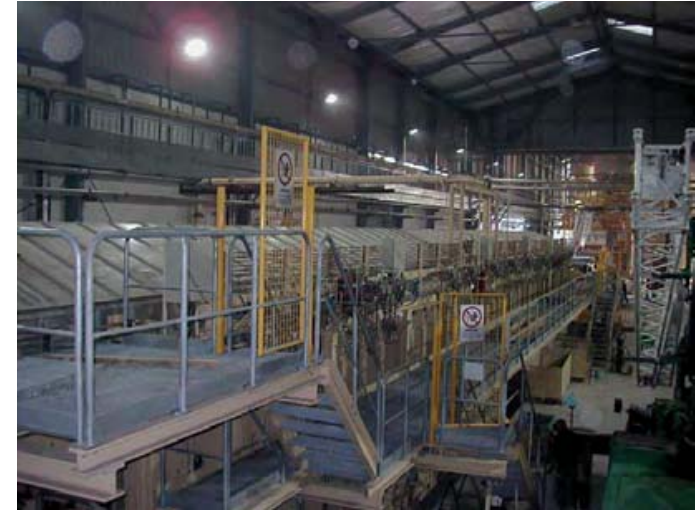
Figure 3.5: Continuous press in a particleboard plant (Sonae Indústria, Oliveira do Hospital plant).
