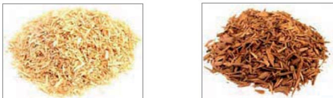
Figure 8.4: Chips of spruce ( Picea abies ) before (left) and after thermal modification.
