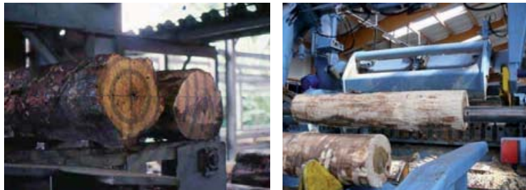
Figure 1.66: Two methods of aligning logs: left a shadow mask and right a laser scan of log as it is slowly rotated.
