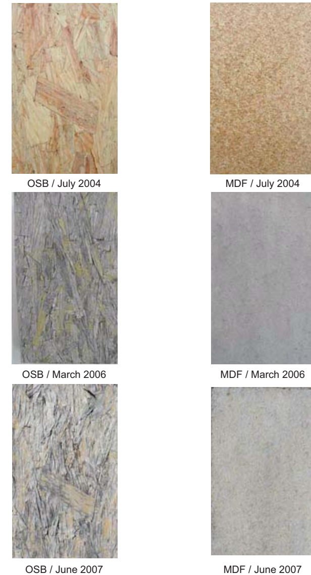
Figure 2.9: OSB and MDF after a natural weathering, (ETH Zurich, IfB, Wood Physics).
