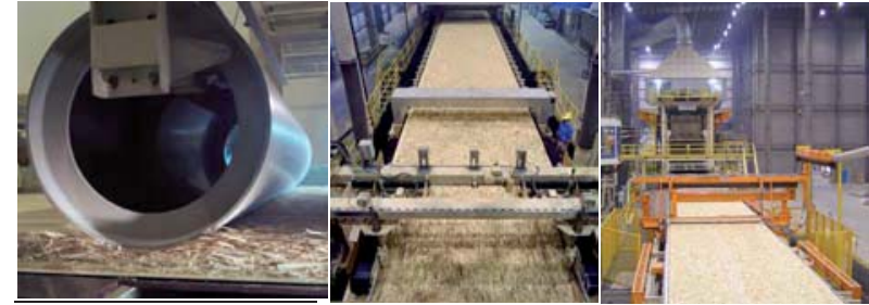
Figure 1.49: An OSB levelling roller as prepress unit and trimming/metal detection in the mattress before pressing in a multidays press (Dieffenbacher).
