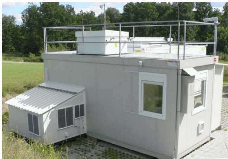
Figure 5.6. The Raman lidar system RAMSES at the Richard-Aßmann Observatory of the DWD in Lindenberg, Germany
