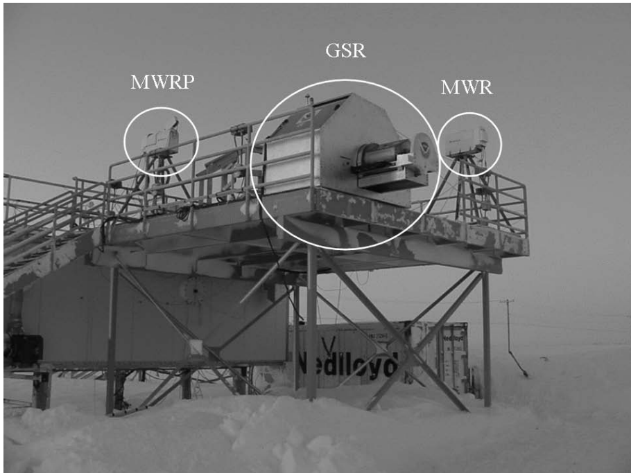
Figure 3.7. Photograph of the deployment of the GSR, MWRP, and MWR at the NSA/AAO Arctic Winter Radiometric Experiment that was conducted in Barrow, Alaska, USA, during March-April 2004.
