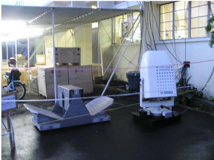
Figure 5.42. Vaisala CT75K lidar ceilometer plus Rutherford Appleton Laboratory 78 GHz fmcw cloud radar (centre of picture) operating in the wet towards the end of the intercomparison
