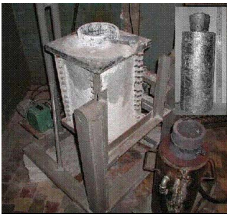
Fig. 5. Overall view of induction furnace and ingot weight ~20 kg.
