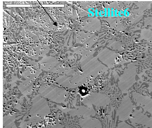
Fig. 11. SEM image near area along the track of Stellite6 hard face coating after tribocorrosion test: 10 N and 30 tours/min, 10000 tours of friction.
