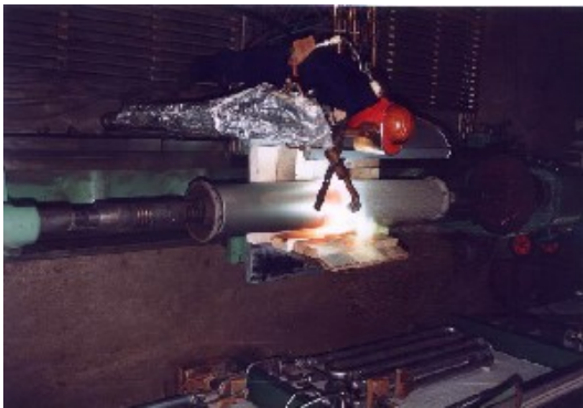
Two steps technology of metal powders spraying (powder NP 62)
