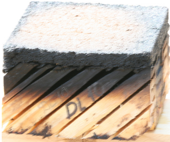
Figure 1: Wood cellular material with mineral and plant fibre coating after reaction to fire tests. Heat flow 50 kW m -2 and test duration 1200 seconds
