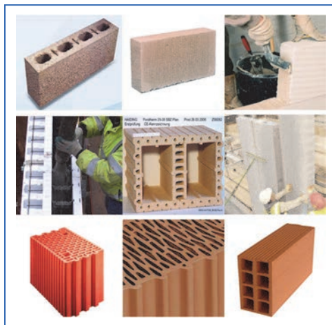
Figure 1.10. Example of masonry and concrete wall types used in European separating walls. (left to right: cellular block, solid block, thin joint aircrete blocks, insulated concrete formwork, large hollow blocks, full height precast wall panels, diverse perforated clay blocks).
