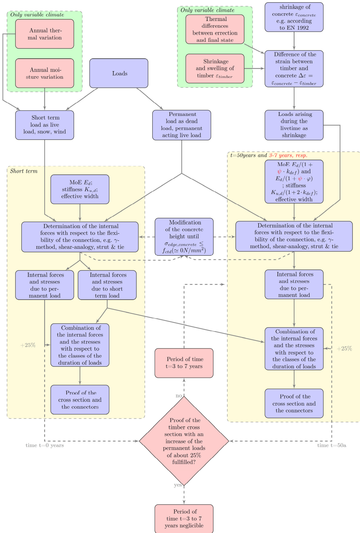
Figure 69: Design process of timber-concrete-composite structures for the ULS
